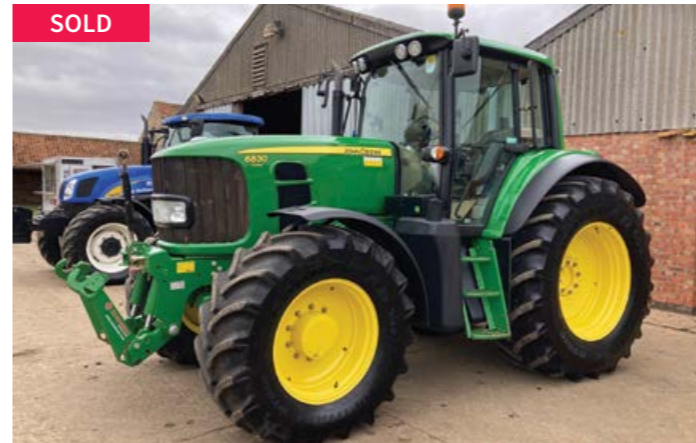
2011 JOHN DEERE 6830 PREMIUM TRACTOR, 40KPH, 24 SPEED, POWER QUAD, WITH FRONT SPOOL & 3 REAR SPOOLS
